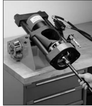
Perfect for maintenance and repair of all your hose needs and designed to be used in remote or portable stations, the ProCrimp 1380P will handle through -20 SAE100R12 hose and fittings. All die cages, crimp diameters and approved hose and fitting combinations are identical to Eaton's popular FT1380 crimper. Crimp diameters are controlled using a micrometer and specially designed hydraulic circuit that allows
