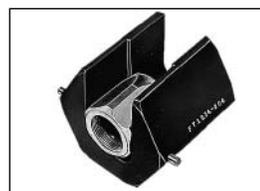
The FT1234 drop-in socket holder is designed for the FT1028 assembly machine. They prevent rotation of the socket during assembly and provide a back stop to ensure consistent location of the socket.
